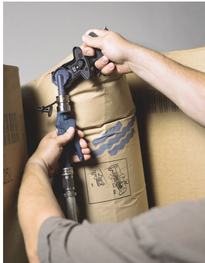
Inflation using quick inflator
