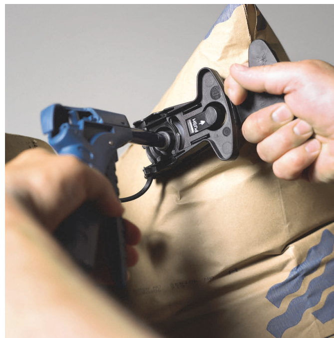
Inflation using standard inflator
